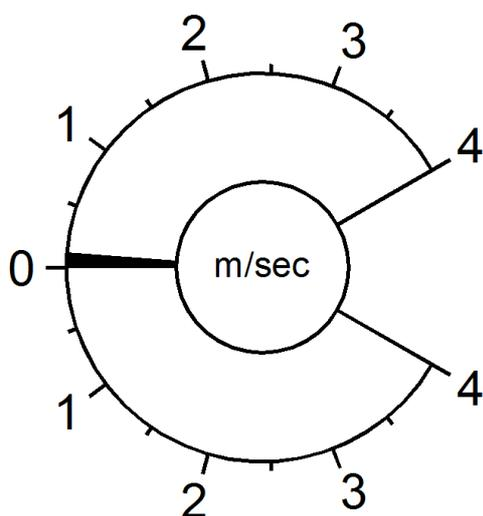
We are in lift of about 1 m/s, approximately equal to the sink rate of our glider. Our vario may be “burbling” or sort of dithering between a lift and sink tones which may also occur whilst stationary at take off. Lift or sink threshold adjustments can be used to create a silent “gap” in the audio to reduce or eliminate this. A setting of about 0.1 to 0.15 m/s is usually about right and ensures that the lift or sink tones are definitely indicating climbing or sinking.
